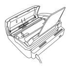
Close the print compartment cover (press down on both sides to make sure it clicks into place), and then close the operation panel.
